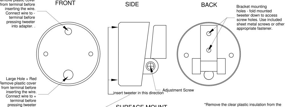
\*Remove the clear plastic insulation from the speaker leads when using this adapter. Wires will not fit through the holes provided and terminals need the extra depth for tweeter to fit completely into adapter.
